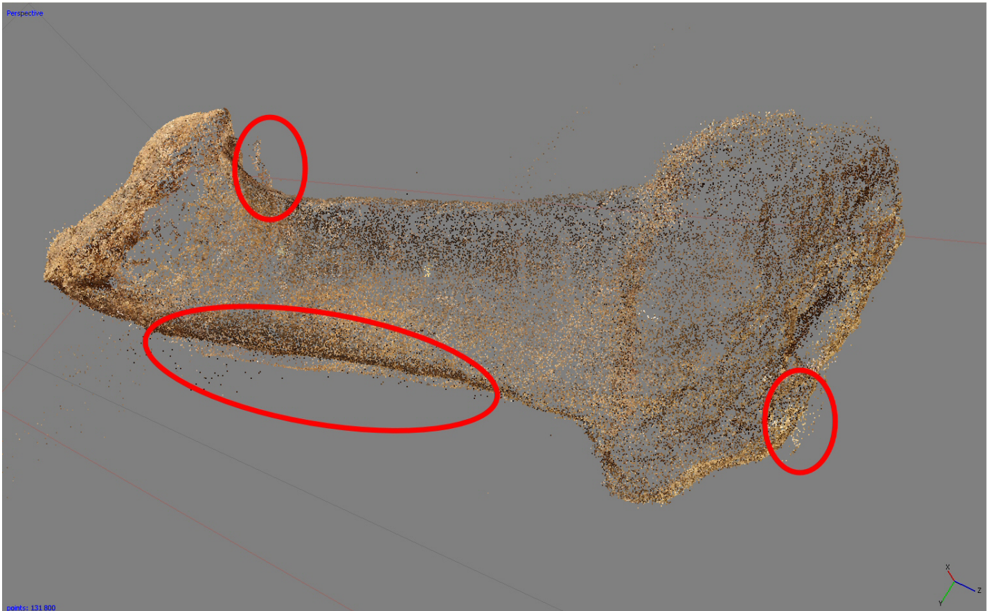
Figure 13: Sparse point cloud from the same image sets as in Figure 12, but computed with the one-chunk method. Comparison to Figure 12 C shows that the one-chunk method here results in a large number of alignment problems. The most obvious resulting erroneous points are circled in red.
